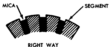
MICA MUST BE CUT AWAY CLEAN BETWEEN SEGMENTS.
